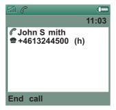
If your network operator provides a CLI (Calling Line Identity) service, your P910i can display the contact's picture together with the other information when an incoming call is received with a CLI matching that contact (not all numbers can be displayed). The contact's picture is also displayed when you make a call to that person.
